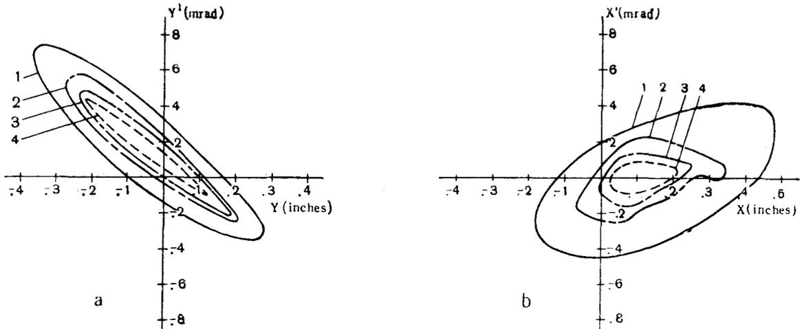
Fig. 9. 50 MeV emittance figures at 10 mA:
