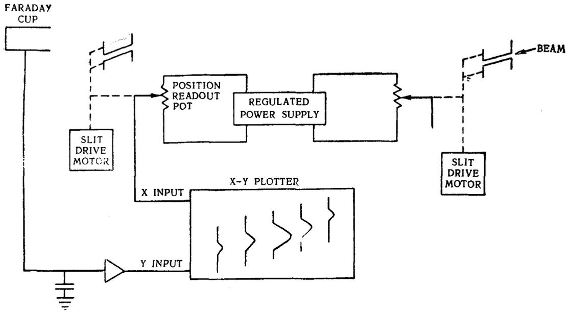
Fig. 8. Schematic of phase space recording equipment.
