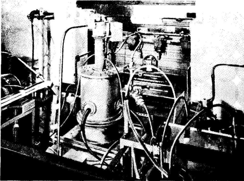
Fig. 6. 200 MHz 5 MW power amplifier.
