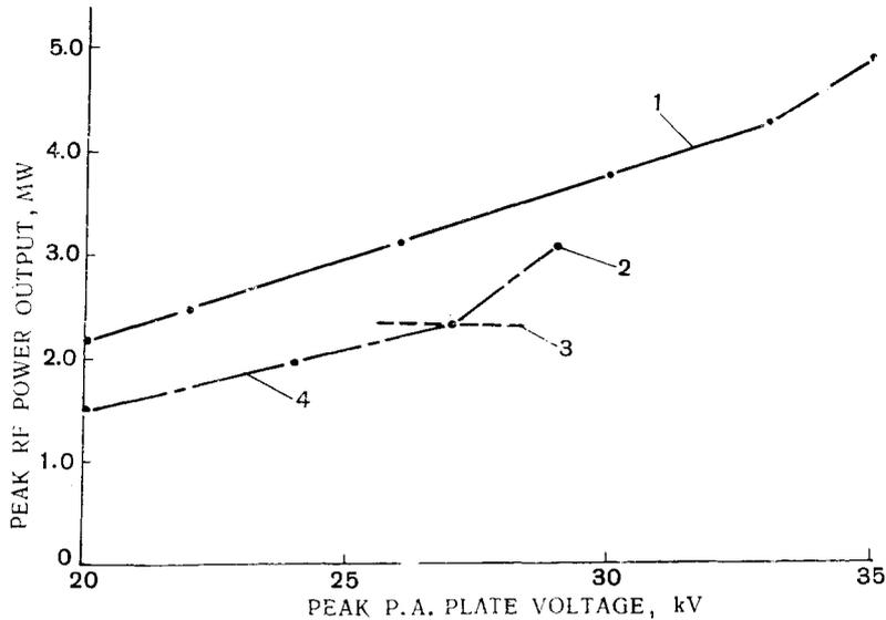
Fig. 5. Measured power amplifier output power vs. plate voltage: 1 — resistive load; 2 — with 10 mA beam; 3 — accelerating gradient excitation power; 4 — power into cavity.
