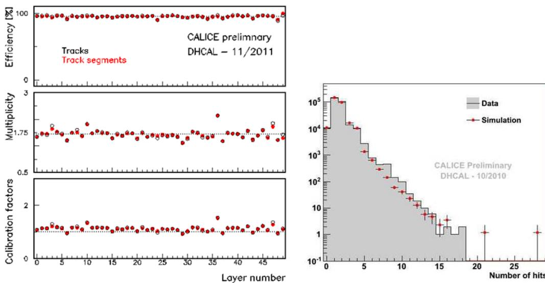
**Figure 2:** RPC performance parameters as function of layer number (*left*). Response to muons averaged over all layers: data (histogram) and simulation (red points) (*right*).
