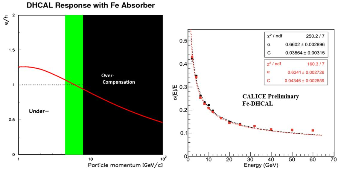
**Figure 4:** Ratio of the response to  $e^+$  and  $\pi^+$  versus beam energy in the DHCAL with Steel absorbers (*right*). Resolution measured with  $\pi^+$  in the DHCAL with Steel absorbers: before (black) and after (red) calibration of the RPC response (*left*).
