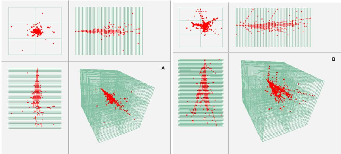
**Figure 1:** Event display of a 8 GeV  $e^+$  in the DHCAL with minimal absorber material (*left*). Event display of a 16 GeV  $\pi^+$  in the DHCAL with minimal absorber material (*right*).
