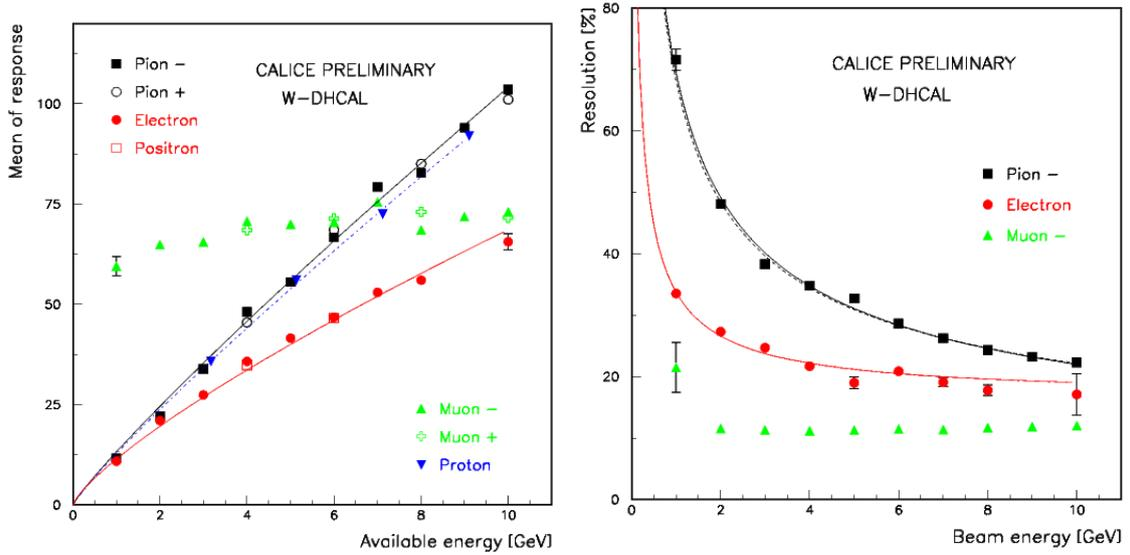
Figure 5: Response measured in the PS beam with Tungsten absorbers (*left*). Resolution measured in the PS beam with Tungsten absorbers (*right*).
