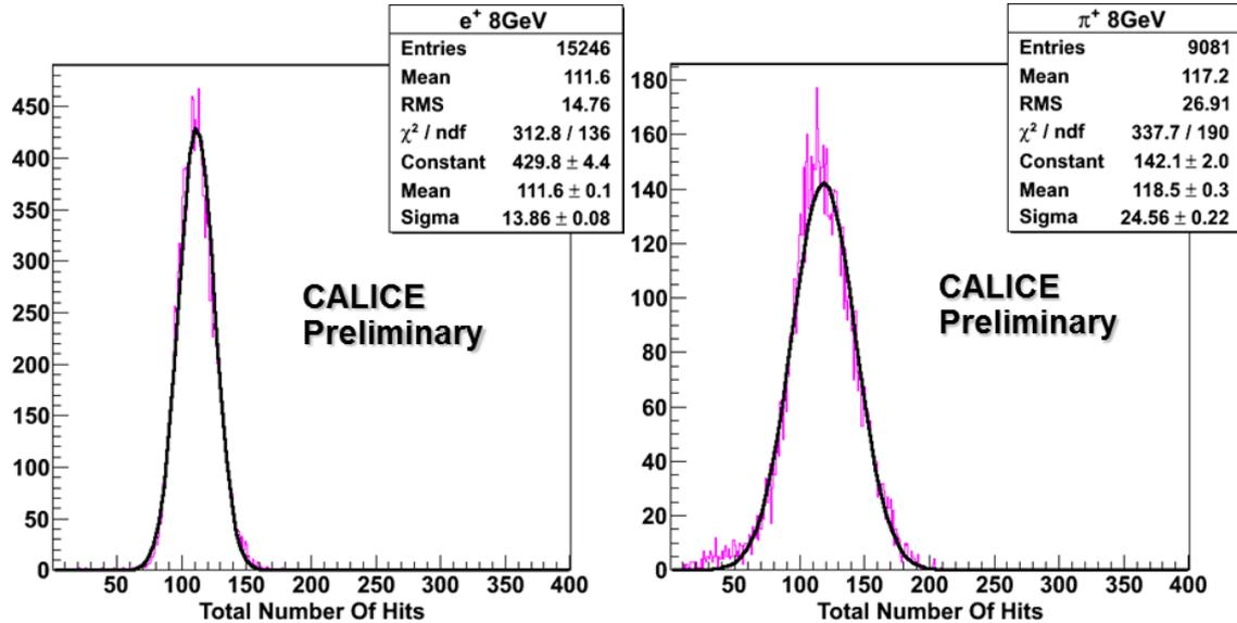
**Figure 3:** Response to 8 GeV  $e^+$  in the DHCAL with Steel absorbers (*left*). Response to 8 GeV  $\pi^+$  in the DHCAL with Steel absorbers (*right*).
