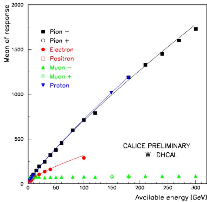
Figure 6: Response measured at the PS and SPS beams with Tungsten absorbers.
