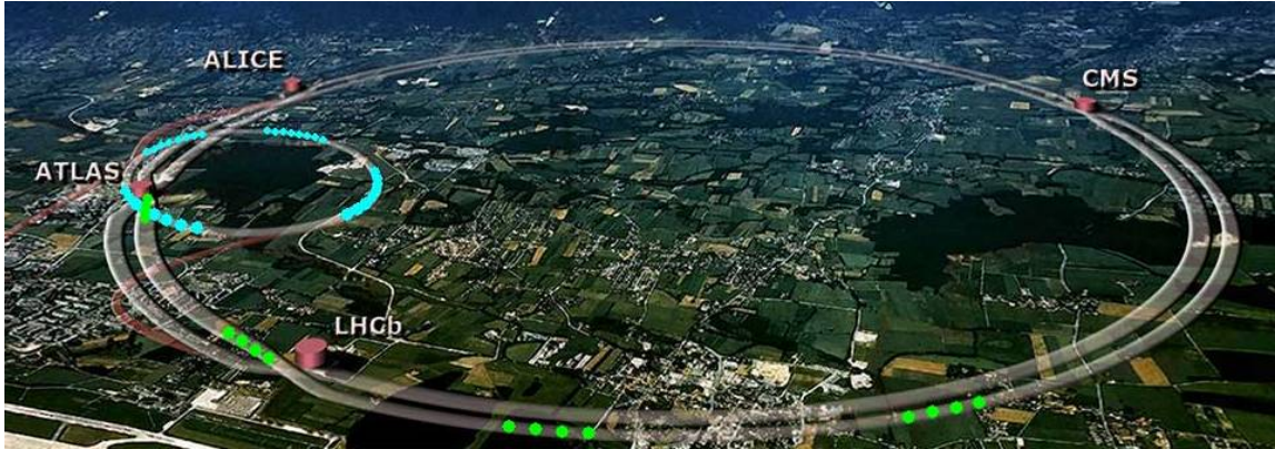
Figure 3.1: Aerial view of the LHC. The two proton beams travel in opposite directions. The four main experiments (ATLAS, CMS, Alice and LHCb) lie along the accelerator's circumference and are located in the interaction regions (IR) where the beams cross.
