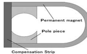
Fig. 2 An example of temperature compensation with compensation material. Compensation strip shunts the flux.
