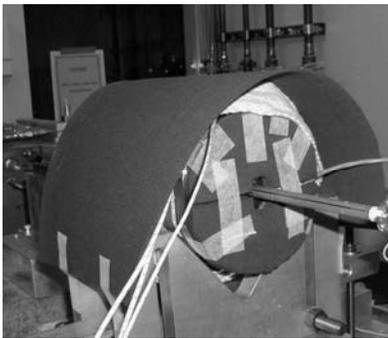
**Fig. 5** PMQ, covered with foam sheet, measured with rotating coil[3].
