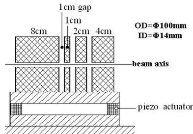
**Fig. 8 Strength Adjustable PMQ.**
