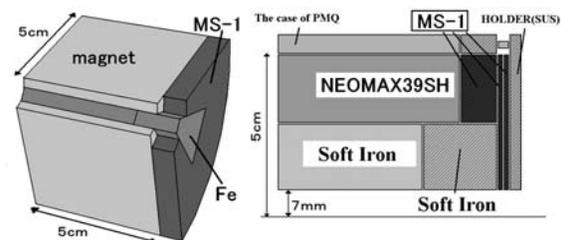
Fig. 3 PMQ with compensation add-on part
