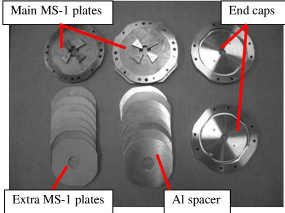
**Fig. 4 Temperature compensation parts**
