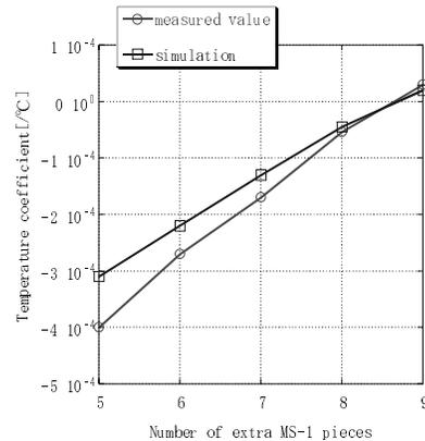
**Fig. 7** Measured and calculated values of temperature coefficient with various numbers of MS-1 plates
