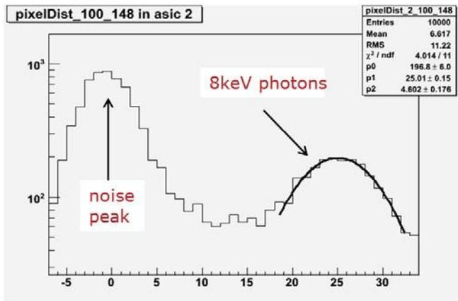
Fig. 7 Measured histogram of a CSPAD-140k pixel illuminated with copper fluorescence in high gain mode
