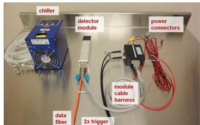
Fig. 1 The full CSPAD-140k kit consists of the detector module with 140kpixels, data fiber, power cable, interface box and a chiller for water cooling.
