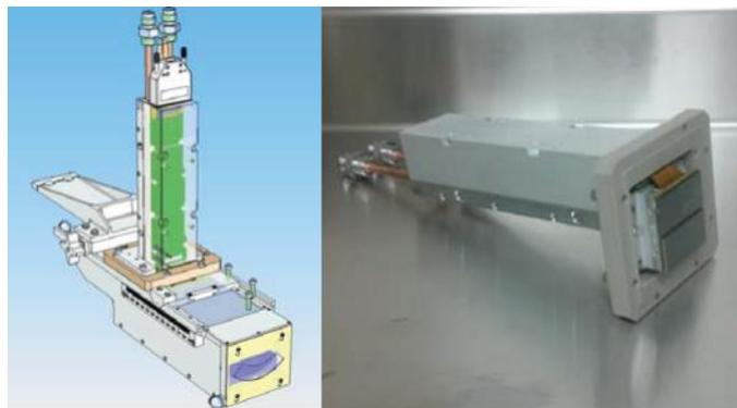
Fig. 3 The CSPAD-140k can be used in a x-ray Thomson scattering spectrometer to substitute a low frame rate CCD with a 120Hz capable detector.
