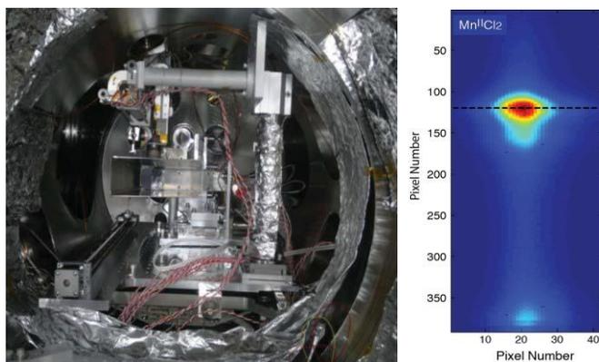
Fig. 2 The CSPAD-140k is used as a detector in a wavelength-dispersive x-ray spectroscopy setup for fluorescence signal analysis during a protein nanocrystallography experiment
