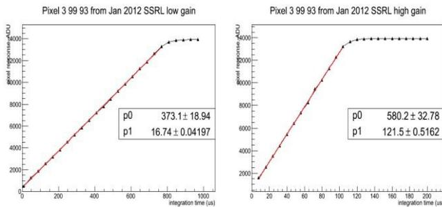
Fig. 6 Linear transfer curve of CSPAD140k measured in low (left) and high (right) gain mode. Different amounts of photons are generated by increasing the integration time with constant illumination conditions.
