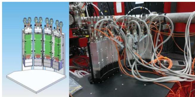
Fig. 5 Multiple CSPAD140k units are combined in an arc like configuration to cover a large angle around the sample.
