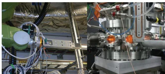
Fig. 4 The compact CSPAD-140k on a robotic arm can be used to measure peak signals in a pump-probe experiment at various positions around the sample chamber. (XPP instrument at LCLS)
