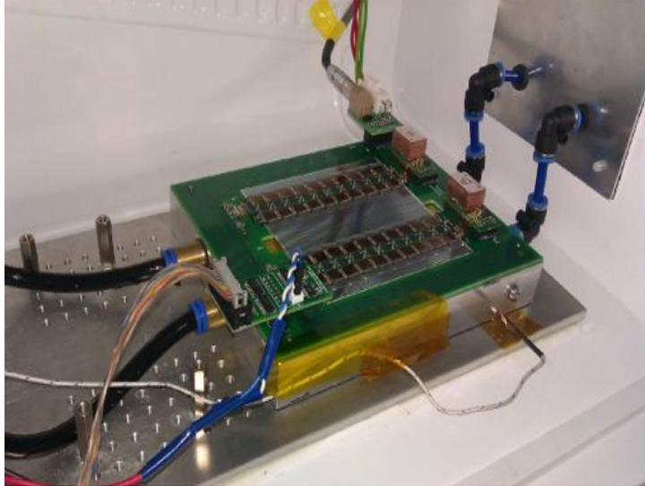
Figure 13.4: Top view of the single-sided DC-DC module placed on a metal jig contained within the fridge.
