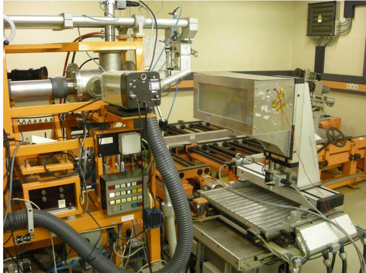
Figure 11.10: Picture of the irradiation setup at Karlsruhe. The miniature sensors are mounted on an aluminium frame and inserted into the insulated box.
