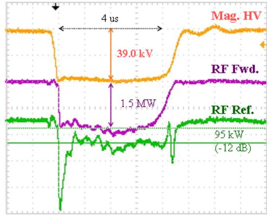
Figure 3: The forward RF power and the reflect RF power at the operating condition.
