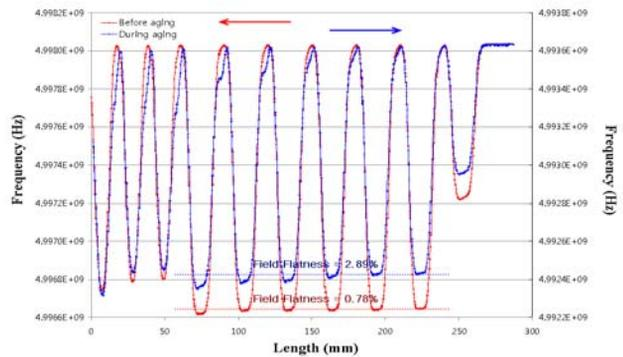
Figure 5: The comparison of the result of the bead test which is conducted before commissioning with during commissioning.
