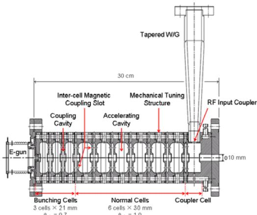
Figure 2: The cross-sectional view of the accelerating structure. The inter-cell magnetic coupling slots are skewed to this plane.
