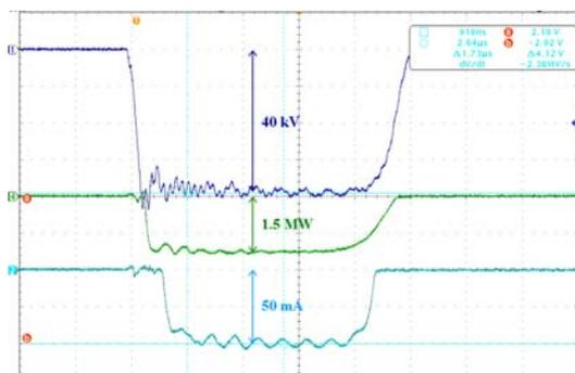
Figure 6: The waveform of the magnetron input high voltage (blue), the accelerator forward RF power (green), and the output beam current (cyan).
