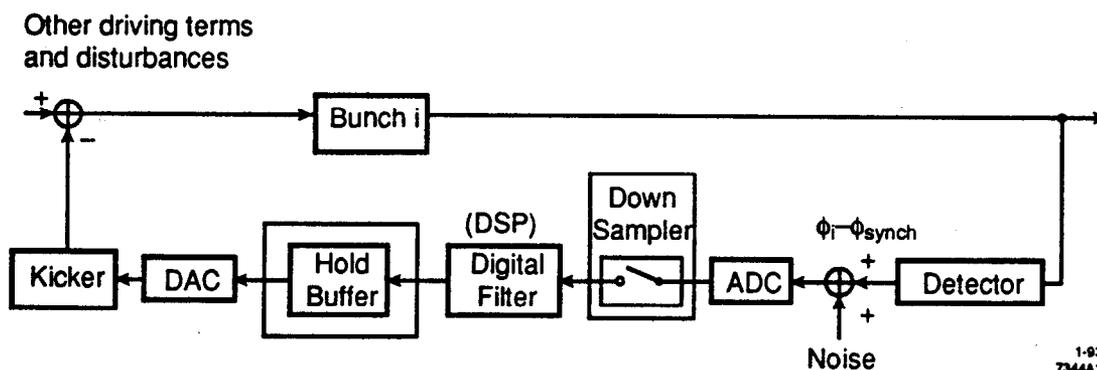
Fig. 1 Conceptual bunch-by-bunch, downsampled feedback system.
