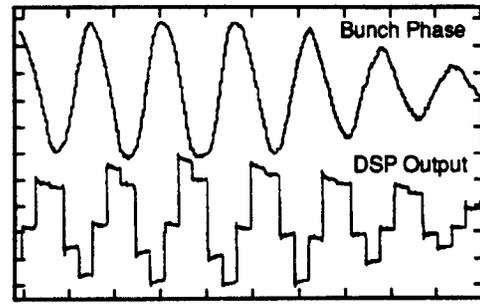
Fig. 9 Filter input and output with downsampling factor of 8.
