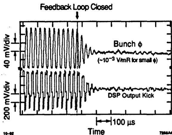
Fig. 11 Time response of an excited bunch and the DSP filter output.
