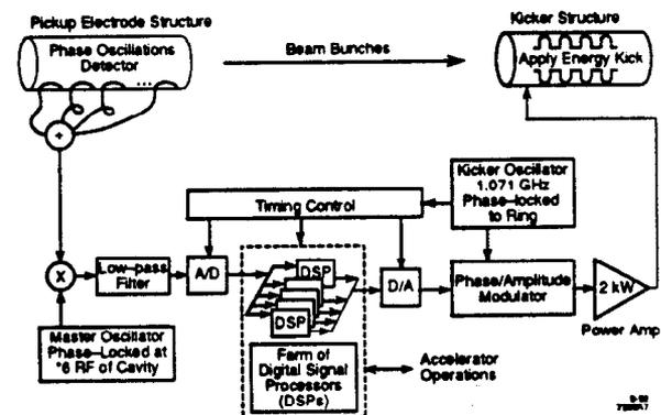
Fig. 2 Longitudinal feedback system without downsampler.
