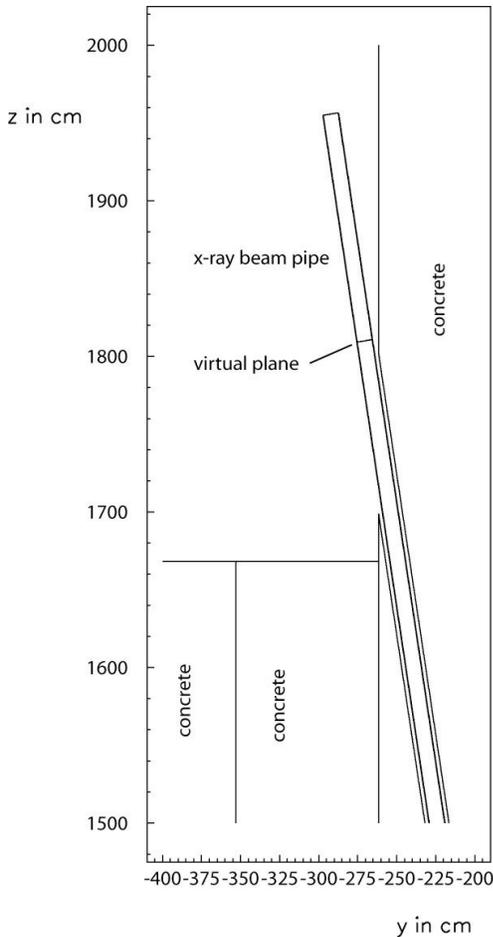
Fig. 5: Details of the FLUKA geometry at the location where the beam pipe exits the FFTB.
