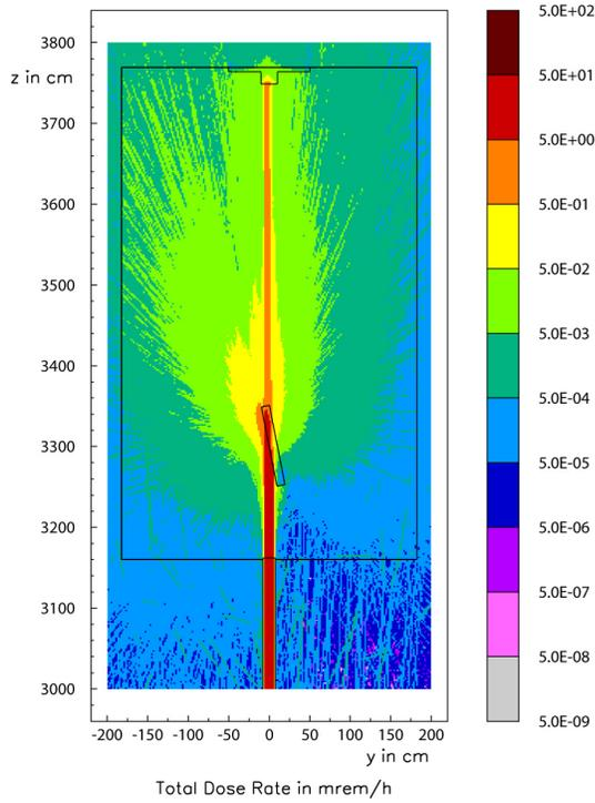
Fig. 12: Case 1 – Total dose rate at the experimental hut. The beam is impinging on a Si-target.
