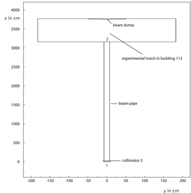
**Fig. 6:** FLUKA geometry of the beam pipe outside the FFTB and the experimental hutch.
