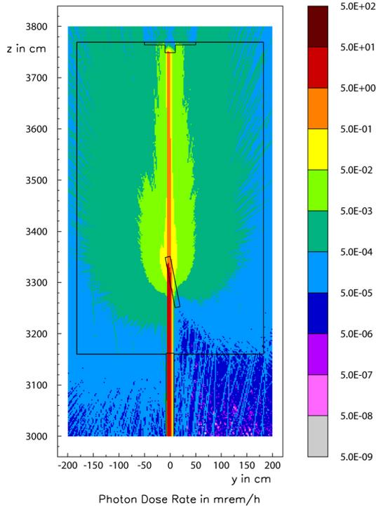
Fig. 13: Case 1 – Photon dose rate at the experimental hut. The beam is impinging on a Si-target.
