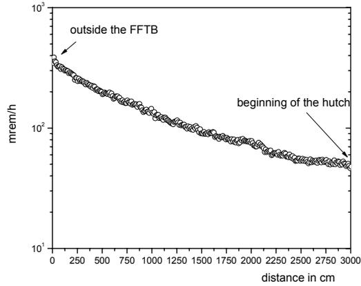
Fig. 8: Case 1 - Total dose rate in the center (1 cm diameter) of the beam pipe
