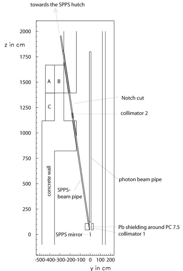
Fig. 4: FLUKA geometry of the FFTB – Horizontal sectional cut at beam height.
