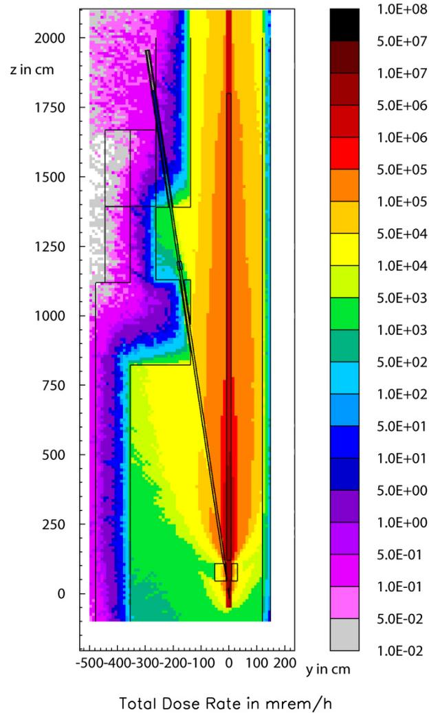
Fig. 7: Total dose rate at the FFTB tunnel
