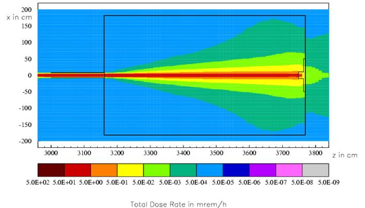
Fig. 11: Case 1 - Total dose rate at the experimental hutch. The beam is impinging on the beam dump downstream the hutch.
