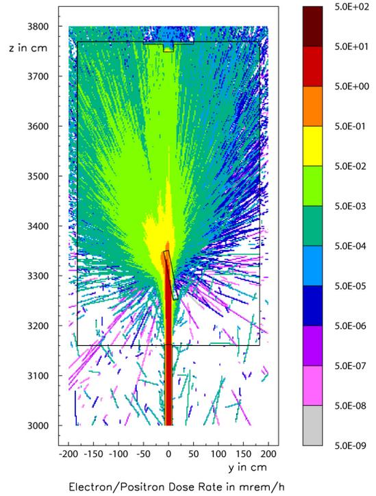
Fig. 14: Case 1 – Electron/positron dose rate at the experimental hut. The beam is impinging on a Si-target.
