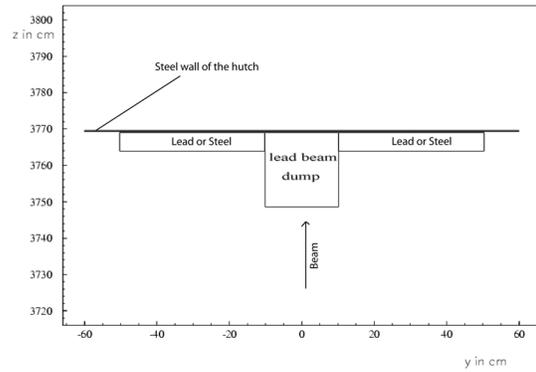
Fig. 10: Horizontal sectional cut through the layout of the beam dump in the experimental hutch in Building 113.
