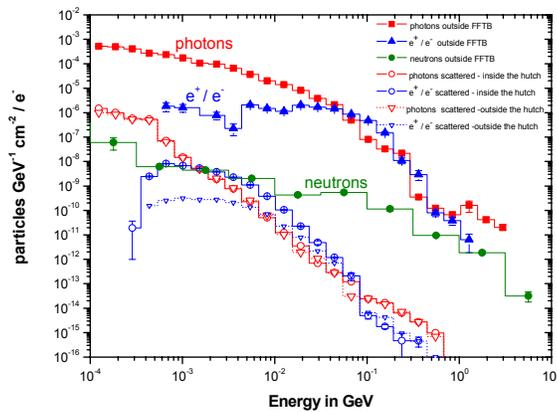
Fig. 17: Spectra of photons, electrons/ positrons and neutrons in case 1 as a function of energy.
