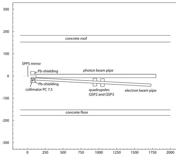
Fig. 3: FLUKA geometry of the FFTB – Vertical sectional cut.
