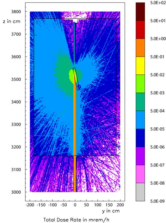
Fig. 16: Case 3 - Total dose rate at the experimental hutch. The x-ray beam is impinging on a Si-target.
