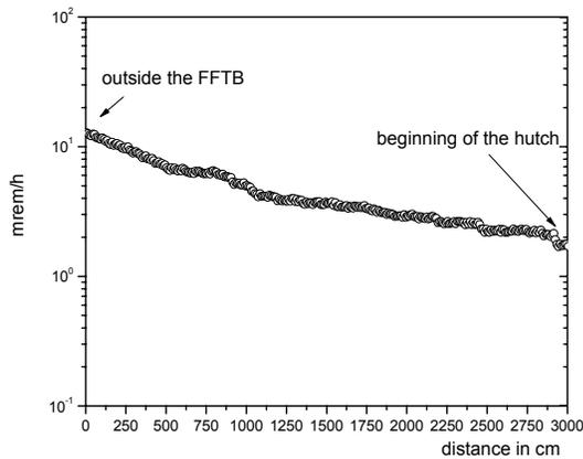
Fig. 9: Case 3 - Total dose rate in the center (1 cm diameter) of the beam pipe
