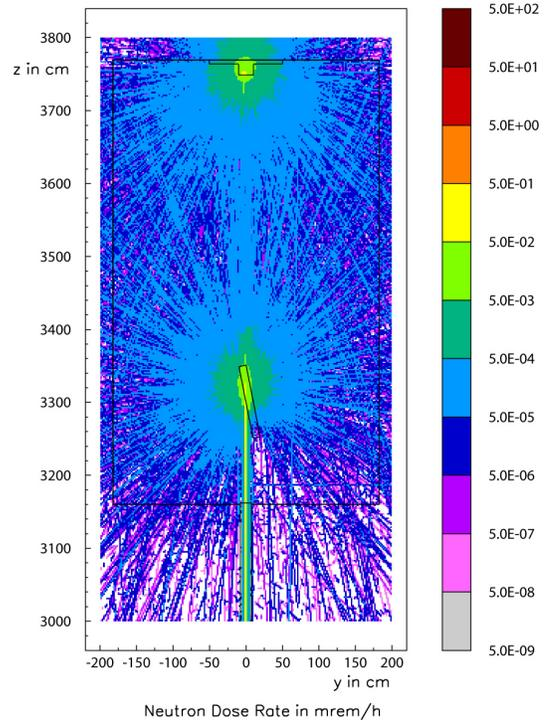
Fig. 15: Case 1 – Neutron dose rate at the experimental hut. The beam is impinging on a Si-target.
