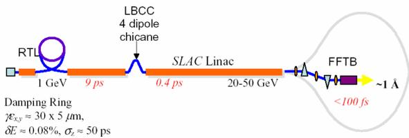
Fig. 1: The e-bunch compression for the SPPS.
