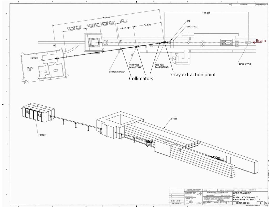
Fig. 2: Layout of the Final Focus Test Beam (FFTB) at SLAC for the SPPS project
