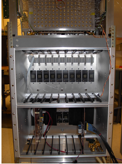
Figure 4.11: Two VME crate “shells” that hold the integrated readout modules on the SciBath detector and align their PMTs with readout fiber bundle cookies (the black rectangles). Also pictured is a board (lower left) that regulates power and clock synchronization signals to the integrated readout modules through a ribbon cable.
