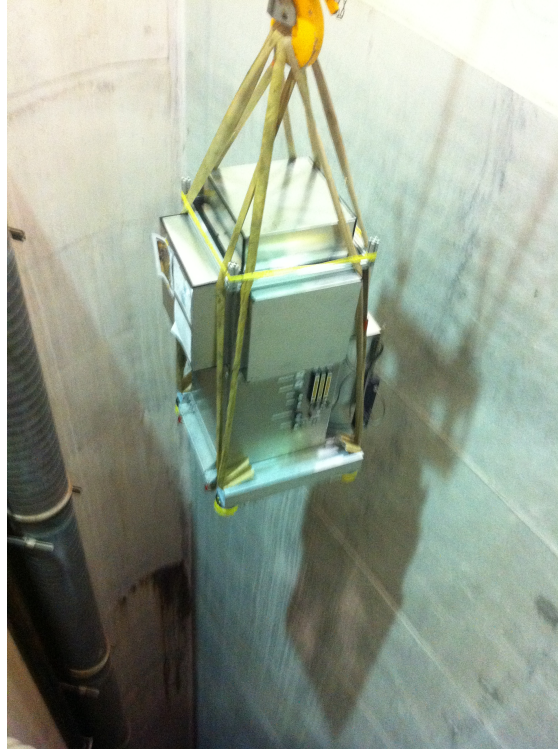
Figure 5.2: The SciBath detector being lowered to the MINOS near detector hall at FNAL.
