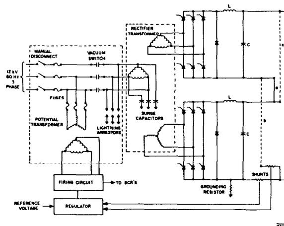
FIG. 1--Elementary schematic diagram of twelve-pulse rectifier power supply.
