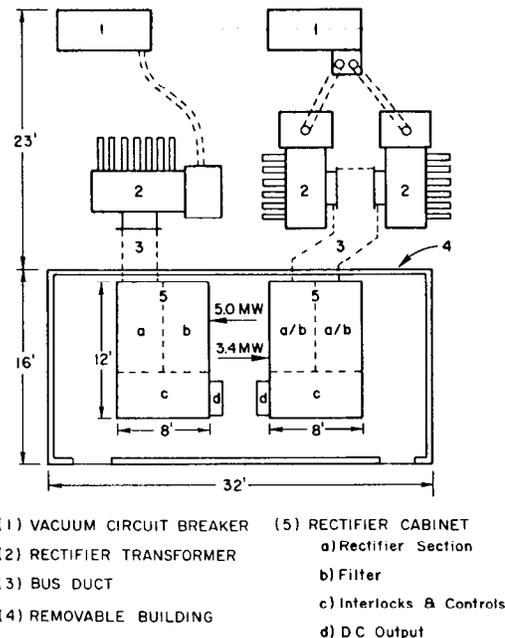
FIG. 3--Plan view of the 3.4 MW and 5.0 MW power supply installation.
