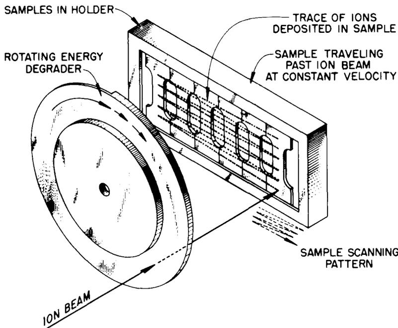
Fig. 3 Irradiation facility for obtaining a homogeneous damage distribution in three dimensions (From ref. 4).
