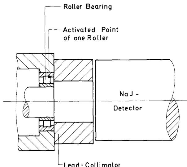
Fig. 7 Apparatus for measuring the speed of revolution of the roller of a roller bearing.
