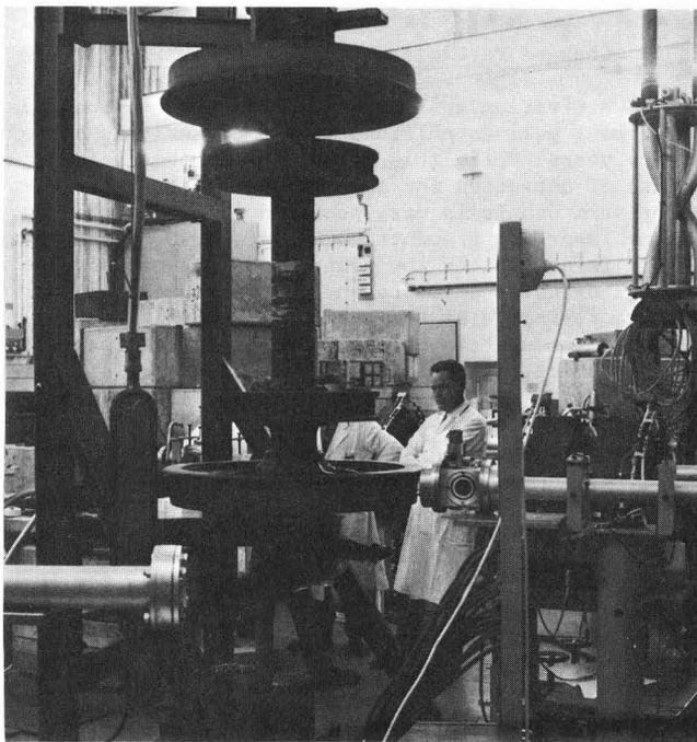
Fig. 5 A set of railway wheels being set up for irradiation at the Karlsruhe Isochronous Cyclotron.
