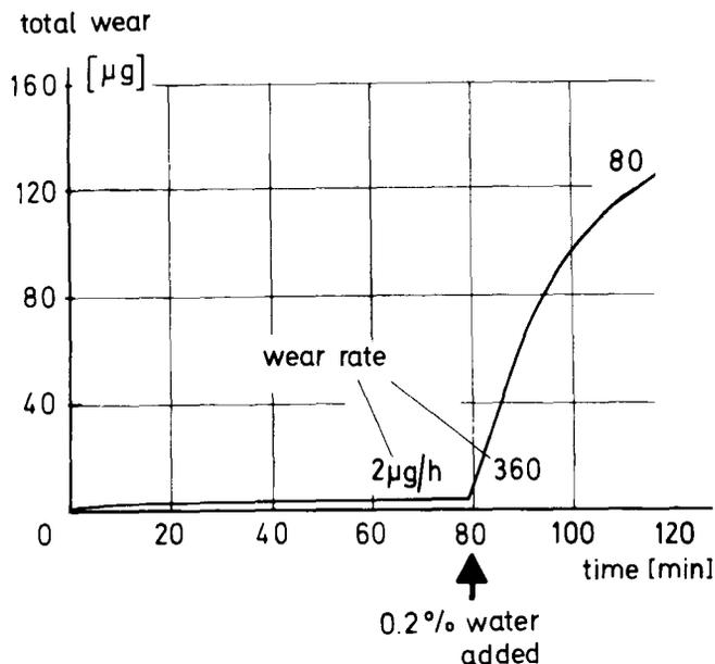
Fig. 6 Measurement of wear on the cage of a ball bearing. At the addition of 0.2 % of water to the lubricating oil the wear rate increases dramatically.
