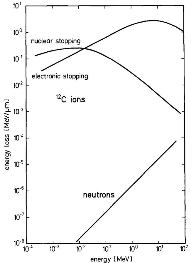
Fig. 1 Average energy loss of <sup>12</sup>C ions and neutrons in nickel. Nuclear stopping data are calculated according to Lindhard et al.<sup>1)</sup>, electronic stopping data are from Northcliffe<sup>2)</sup>. For neutrons, a total scattering cross section of 5 barns and isotropic scattering has been assumed.
