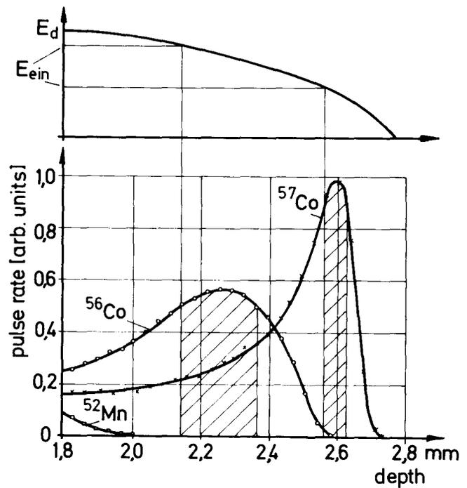
Fig. 4 Upper part: Energy versus penetration depth for a charged particle beam. Lower part: depth distribution of activity produced by 52 MeV deuterons in iron. The hatched area indicates the part of the range most useful for wear studies. The upper part indicates how the corresponding particle energy is determined.
