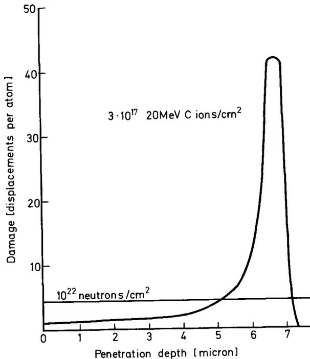
Fig. 2 Depth distribution of radiation damage by <sup>12</sup>C ions and fast neutrons in nickel. Note the difference in the number of incident particles. (Redrawn from ref. 3).
