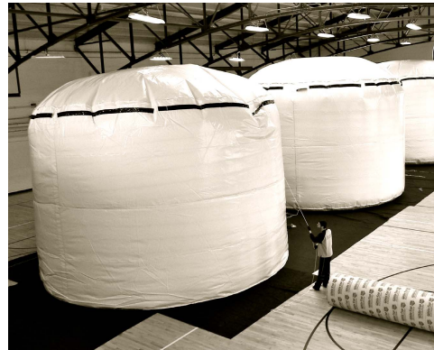
Figure 2: CSU bladders being tested for light leaks.
