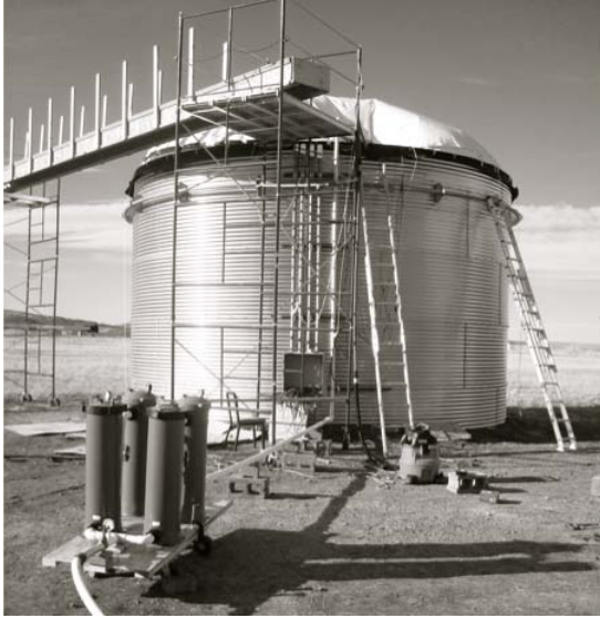
Figure 1: WCD prototype at CSU being filled with water.
