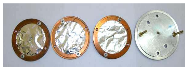
Fig. 10. Beam spot sizes on Al foils and Al collector disk.
