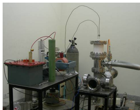
Fig. 7. Electron gun on DP based test bench (left) and on the TMP based test bench (right).
