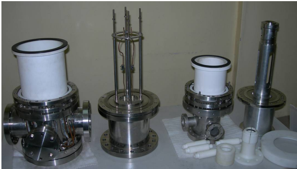
Fig. 6. Comparison of electron gun sizes. The right one is the gun for the 6 MeV linac.
