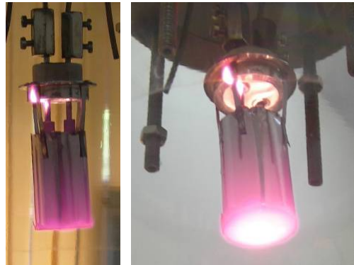
Fig. 12. Large filament current flow (30 A) through the Ta rod and Ta strip due to internal shorting of the filament with the body.
