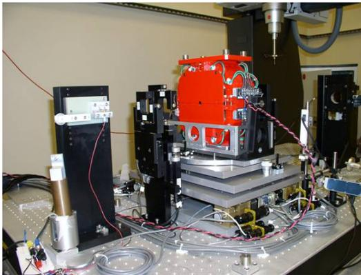
Figure 5: Quadrupole fiducialization system using a vibrating wire and a coordinate measuring machine.
