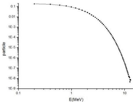
Figure 1: The photon spectrum of synchrotron radiation.
