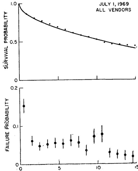
Fig. 4—Klystrons survival and failure probability.
