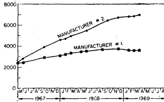
Fig. 6.— Average lifetimes of failed thyratrons.
