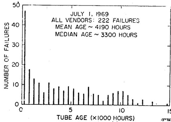
Fig. 3—Failed klystrons age distribution in 500-hour increments.
