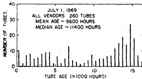
Fig. 2.—Operating klystrons age distribution in 500-hour increments.
