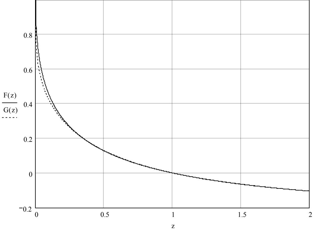
**Figure 1:** The exact and the approximate IBS functions for a round beam.
