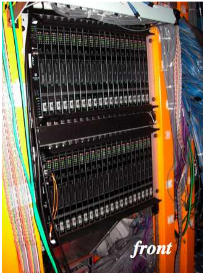
Fig. 3. The new track finding hardware installed under the DØ detector. The 40 new DFEA2 boards are arranged in 2 crates, easily accessible from the front. The 320 input and 320 output cables are located in the back of the crates.
