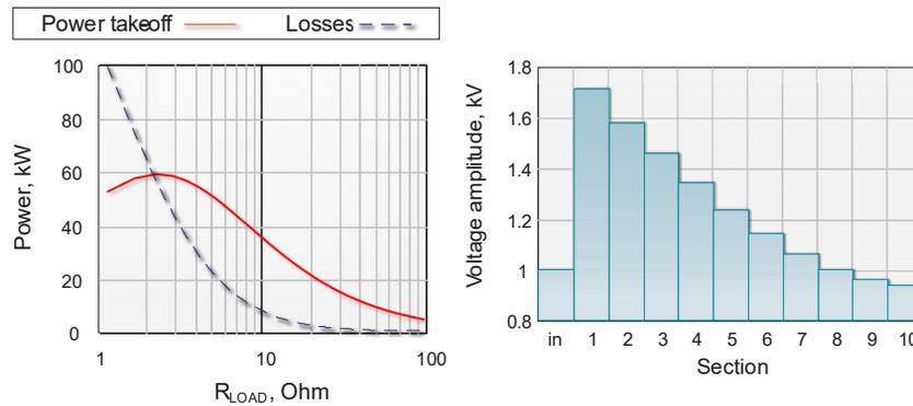
Figure 8: Transfer function of cascade transformer with compensative capacitor  $C_s = 180$  nF from one side.
