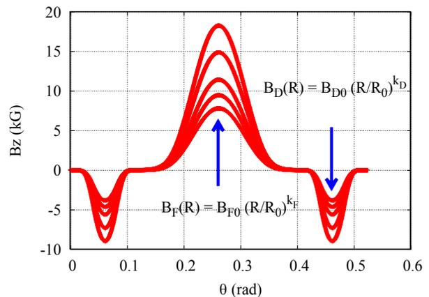
Figure 1: Magnetic field along several closed orbits.
