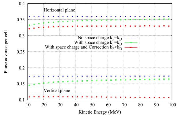
Figure 6: Phase advance per cell before and after perturbation of the average field index of the D-magnet: before correction  $(k_F, k_D) = (7.6, 7.6)$  while after correction  $(k_F, k_D) = (7.6, 7.11)$ .
