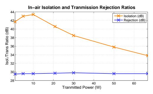
Figure 5-6: The measured isolation and transmission rejection ratios as a function of power. The isolation ratio is defined in equation (5-2) and the transmission rejection ration in (5-3) respectively. These measurements were made in air, and at the time the Faraday isolator was optimized at 20 W of input power.
