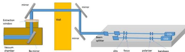
Figure 1: Optical set-up of the TPS SRI system at the 40th beam port.
