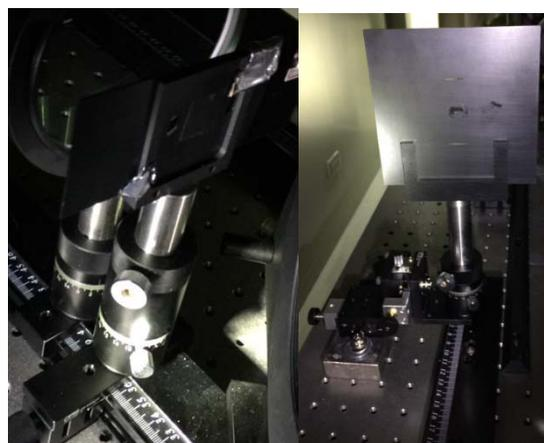
Figure 5: The double slit is supported by two types of mechanisms. (A) Method A: The slit holder is fastened on a single rod with a damping pad. (B) Method B: The slit holder is installed on a stage with two axis adjustments.
