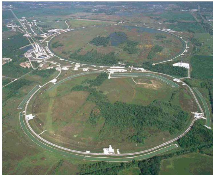
Figure 2.1: Aerial view of the accelerator complex at the Fermi National Accelerator Laboratory. The upper ring is the Tevatron, and lower is the main injector.
