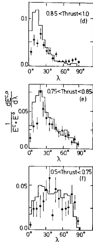
Fig. 21. PLUTO Collaboration: Angular distribution  $1/E dE/d\lambda$  of neutral (data points) and charged (histogram) energy with respect to the thrust axis for three different thrust intervals.  $\lambda$  is the angle between the momentum vector and the thrust axis.
