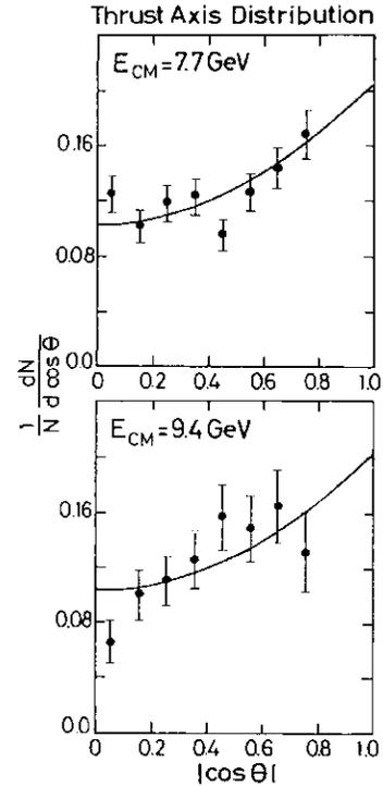
Fig. 20. PLUTO Collaboration: Angular distribution of the jet axis as defined by thrust for two energies.
