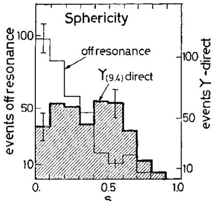
Fig. 26. DESY-Hamburg-Heidelberg-Munchen Collaboration: Observed sphericity distribution for events on and off resonance in the  $Y$  region. The sphericity is defined from the measured shower energies.
