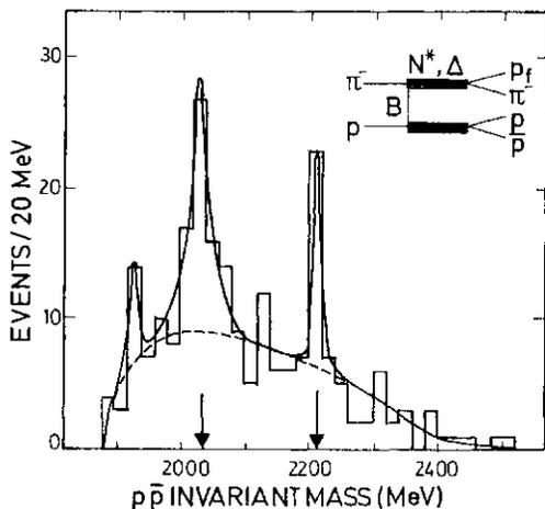
Fig. 3. CERN-College de France-Ecole Polytechnique-Orsay Collaboration: Backward ( $pp$ ) mass distribution in the reaction  $iz\sim p\rightarrow\%ppp$  exhibiting two narrow peaks at 2.02 and 2.20 GeV, 9 and 12 GeV data with selection on  $\hat{a}$  and  $\cos\theta^*(p,p) < 0$  are shown.
