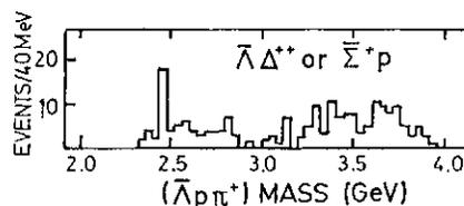
Fig. 4. Glasgow-DESY Collaboration: ( $Apn$ ) mass distribution in the reaction  $K+p\sim^Apn$  with an indication of a peak at 2.46 GeV.
