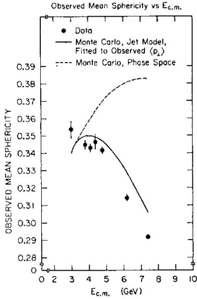
Fig. 18. SLAC-LBL Collaboration: First evidence for jets in  $e^+e^-$  annihilation. Observed mean sphericity as a function of energy. The full and dashed lines show Monte-Carlo simulations of a jet and phase space model, respectively.
