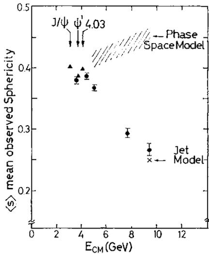
Fig. 19. PLUTO Collaboration: Observed mean sphericity of charged particles ( $>4$  prongs) as a function of energy. The shaded region represents the phase-space prediction, the crossed one for two jets.
