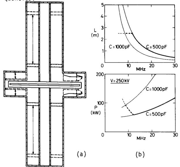
Figure 4. (a) Cross-sectional view of a resonator with movable short-circuit plates and two types of capacitance variation. (b) Variation of the length of each transmission line (L) and power loss (P) as a function of frequency for different values of delta capacity.
