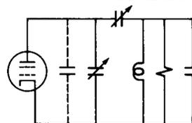
Figure 7. Simplified diagram of an amplifier directly coupled to a resonator.
