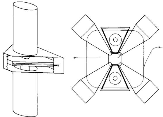
Figure 2. A half-wave delta resonator and the positioning of two of them in the OSC.
