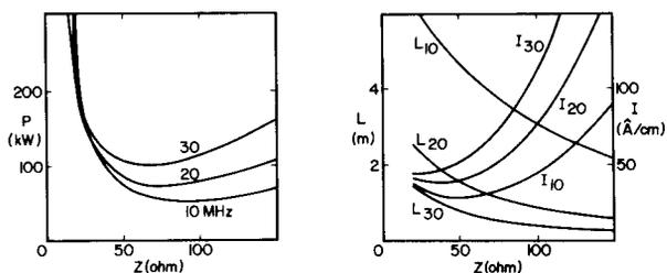
Figure 5. Variation of energy loss (P), peak current density (I) and length of each transmission line (L) as a function of the characteristic impedance (Z) of the lines, using a fixed outer diameter at three different frequencies (i.e. 10, 20, and 30 MHz).
