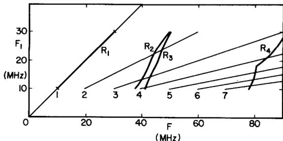
Figure 6. The relation between the required frequencies ( $F_1$ ) and the resonance frequencies ( $R_n$ ) obtained from the measurements on a model. The thin lines (2 to 7) represent harmonics of the required resonance frequencies ( $R_1$ ).
