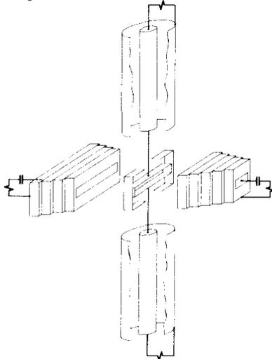
Figure 3. The model used for the calculation of the characteristics of a half-wave delta-resonator.
