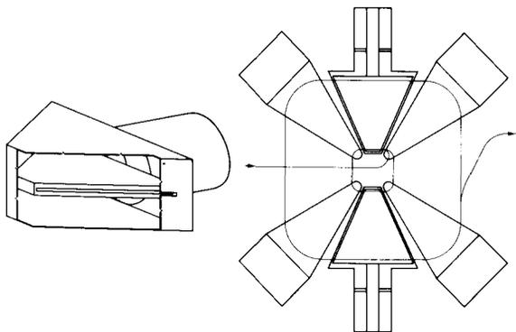
Figure 1. A quarter-wave delta resonator and the positioning of two of them in the OSC.
