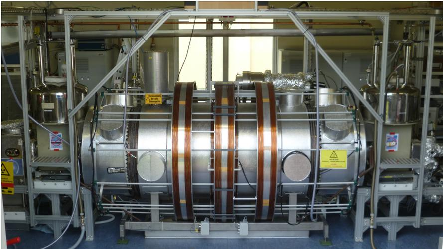
**Figure 2.8:** Monitor spectrometer, installed at the KIT site. Two solenoids and 4 air coils (3 visible, 4<sup>th</sup> hidden by the middle one) produce the magnetic guiding field.
