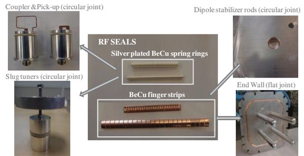
Figure 3: RF seals tested including dipole rods.
