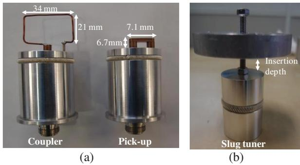
Figure 2: (a) Coupler and pick-up; (b) slug tuner.
