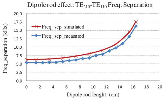
Figure 5: Dipole stabilizer rods effect.
