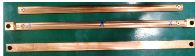
Figure 7: Blades of strip-line kickers.
