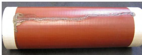
Figure 4.29. A high voltage resistor damaged during processing.
