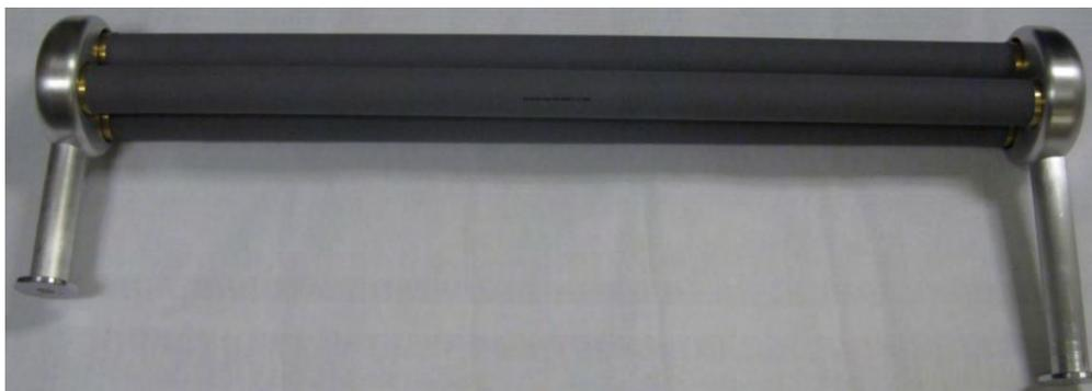
Figure 4.30. Processing resistor schematic using three long resistors in parallel.
