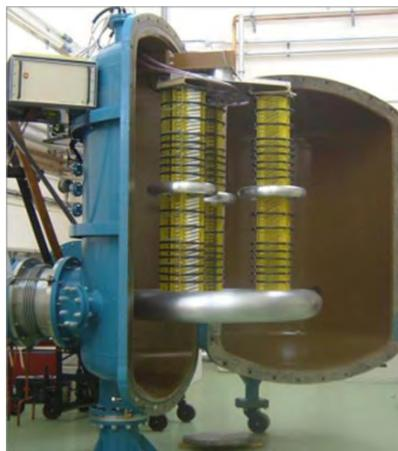
Figure 4.25. 500 kV, 8 mA power supply (Glassman HV, Inc.) and  $\text{SF}_6$  tank used at Daresbury Laboratory [4.54]. [Credit to ASTeC, STFC Daresbury]
