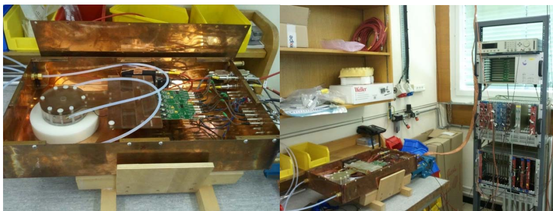
Figure 5.16: The Faraday cage and the position of the detector on the test bench (left) and the complete calibration system (right).
