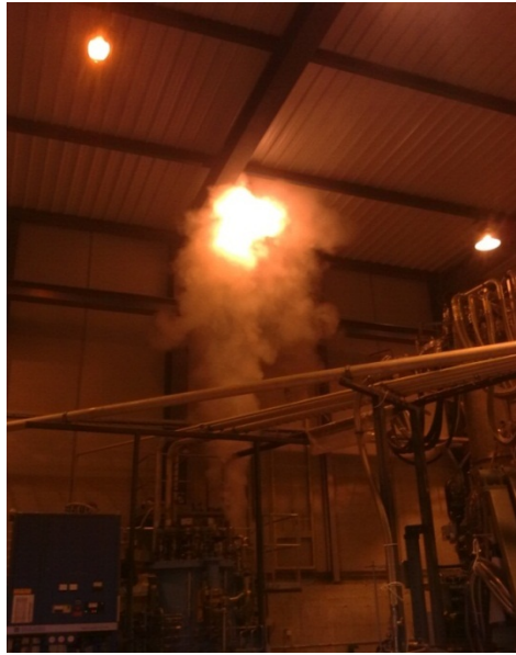
Figure 2.7 A quench in the CAST magnet. The liquid helium starts boiling and is evacuated through exhaust pipes in the atmosphere.
