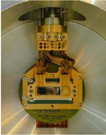
Figure 2.27: Left: The pn-CCD detector. The rectangular pn-CCD chip is visible in the centre, surrounded by the gold plated cooling mask. Right: The Quantum Efficiency of this type of detector is close to 90% for the region of interest of 1-7 keV.
