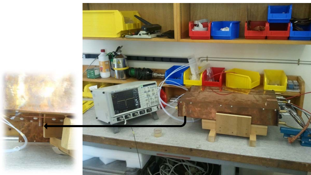
Figure 5.17: The Faraday cage is closed during a calibration for minimizing the noise (right). The socket in which the radioactive source is placed, on the bottom side of the Faraday cage (left).
