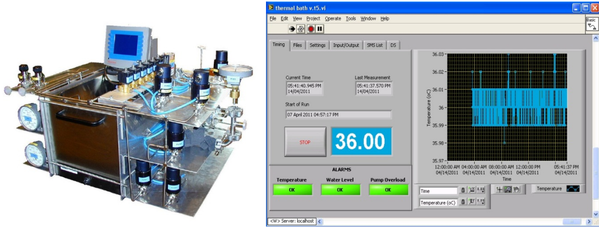
Figure 2.22 The thermostatic bath (left) keeps the Metering Volumes at a constant temperature to ensure reproducibility and high precision. Since the constant temperature of the bath is of high importance, control software was developed (right) to monitor and alarm for possible malfunctions of the device.
