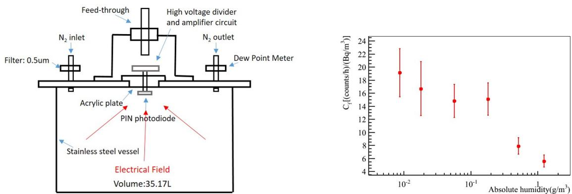
**Figure 2.** Left: the scheme of radon detector. Right: absolute humidity dependence of the calibration factor.
