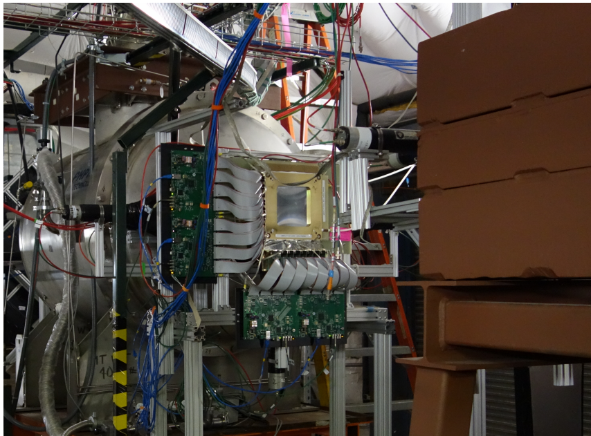
Figure 6. One of the multiwire proportional chambers in the LArIAT tertiary beamline.
