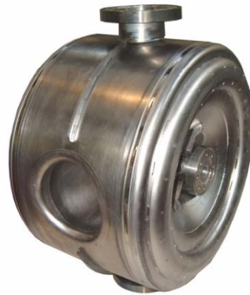
Figure 1: The first completed SSR1.
