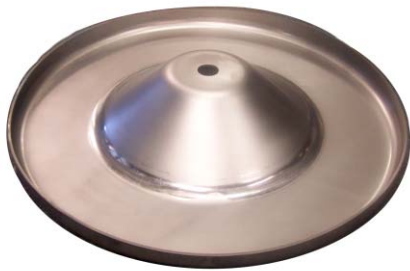
Figure 3: The SSR1 end wall stamped from a single sheet.
