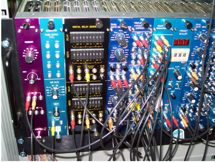
Figure 3.28: A photograph of the NIM modules used in the SN Burst test which the author of this work arranged to simulate a SN signal.
