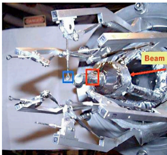
Fig. S9: The EG2 target. The red square shows the center of the \text{LD}_2 target cell. The blue square shows the solid target. The red arrow marks the approximate beam direction. As can be seen, the beam passes throughout both targets simultaneously.
