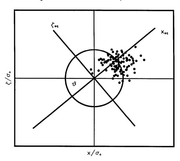
amplitude functions are written in units of the natural amplitude function of the synchrotron  $\beta_2 \equiv \beta_0 \equiv 1$ . In addition, the particle distribution is normalized to one particle, i.e., N = 1. Injection Position Mismatch
