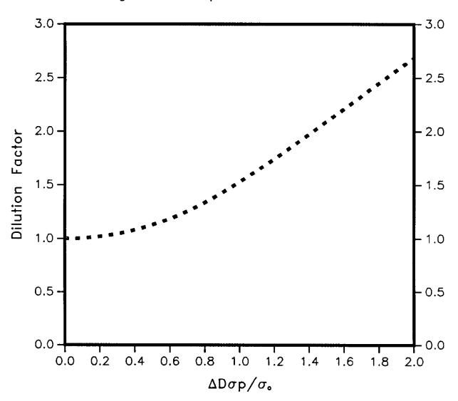
size would not increase no matter how large a value for  $\Delta D$  is obtained. Likewise, any small deviation from the ideal dispersion function significantly affects the emittance of a beam which has a large enough momentum spread. Even for values of  $\Delta D\sigma_{\bf p}$  as large as 1.5, the variance of the resulting time average distribution provides a good estimate of the dilution factor Fp.
