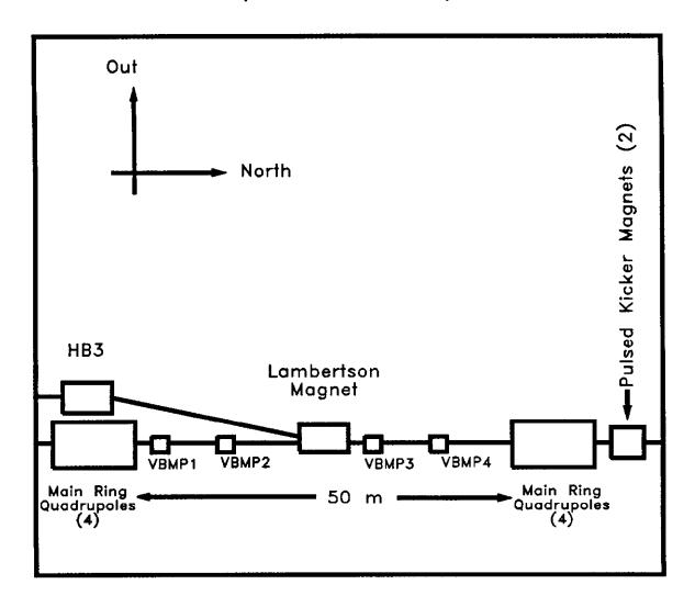
chosen for the orbit bump are those which had been used in the Fermilab Electron Cooling project.  $^3$  These magnets have 40 turns, apertures of 3 in. x 12 in., and lengths of 48 in.
