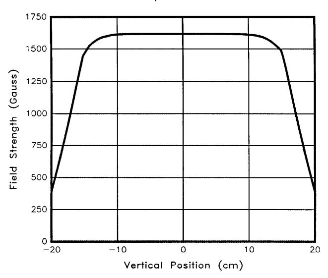
problem with the orbit bump magnets was identified and understood, they were replaced with dipoles of much higher quality. These new magnets were described in Chapter IV and their calculated bend field is shown in Figure VI-2. A more detailed account of the effects which the original magnets had on the circulating Main Ring beam is provided in the Appendix.
