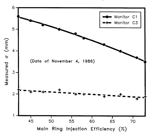
One such plot is shown in Figure VI-5. From this particular graph, the horizontal normalized emittance and the variance of the momentum distribution may be read. By allowing the plot to update over an extended period of time, the uncertainties in these two quantities may be obtained easily. (For Figure VI-5, roughly 200 points were obtained.)
