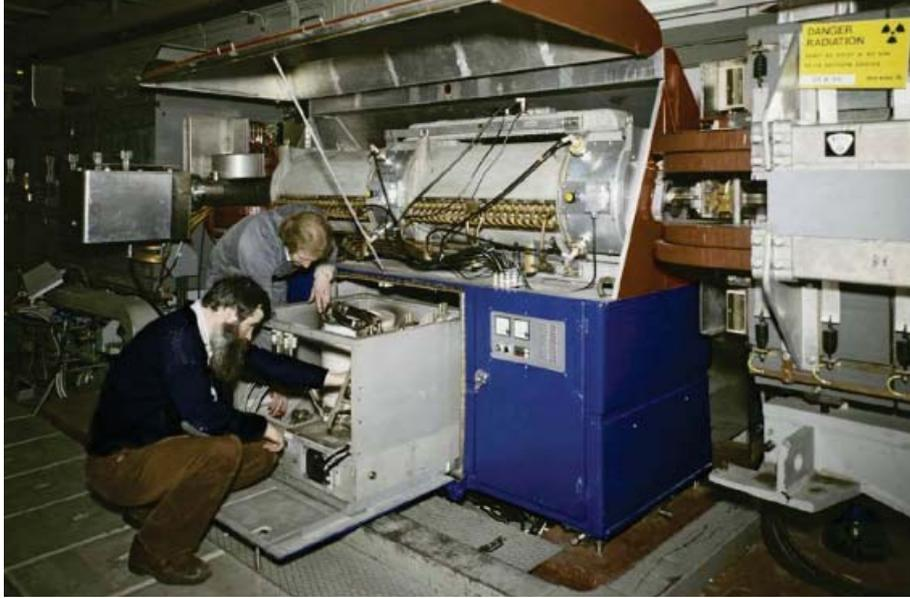
**Figure 5.5.** On of the CERN PS 10 MHz cavity
