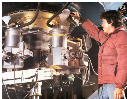
Figure 1. — A youthful Jay Tsutsumi tops up the liquid nitrogen in UKT6 at the Cassegrain focus of UKIRT (c. 1982). UKT5 can be seen to its left. (Image courtesy Royal Observatory Edinburgh.)
