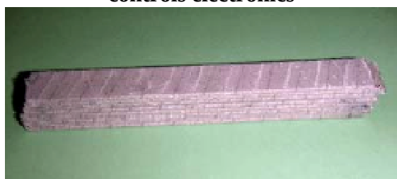
Cable stack with ceramic insulation
