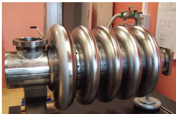
Prototypes of superconducting accelerating structures and components. From left, elliptical cavity B, spoke cavity, prototype coupler.
