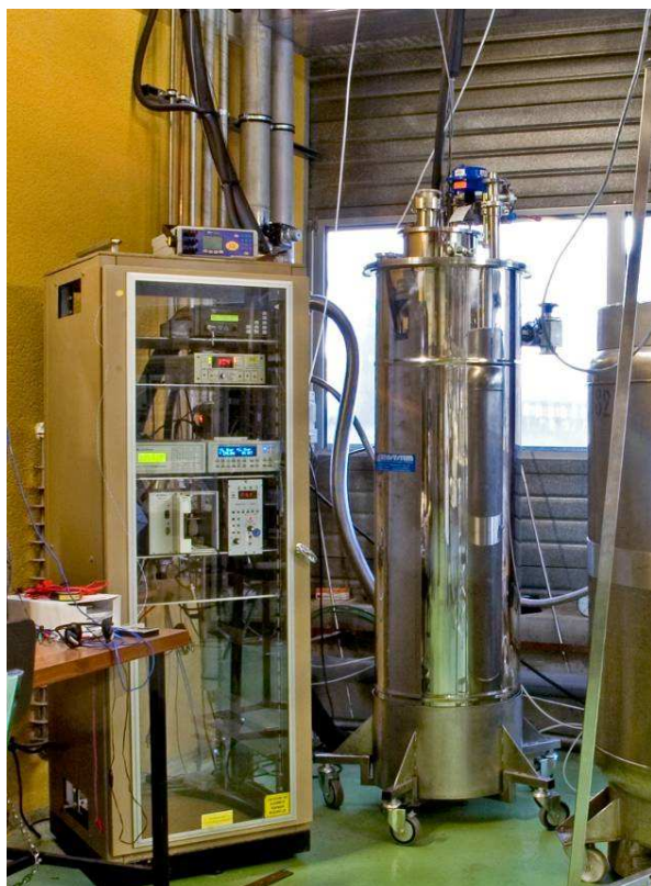
Heat transfer studies cryostat and controls electronics
