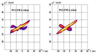
Figure 4: Emittance gain by injecting N<sub>2</sub> gas into the SILHI beam line.
