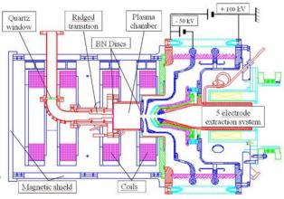
Figure 3: SILHI source design with BN disks, Electron repeller, Window protected by a bend, Ridged waveguide transition
