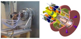
Figure 6: Picture and 3D view of the Spiral 2 ion source with permanent magnets and 5 electrode extraction system.
