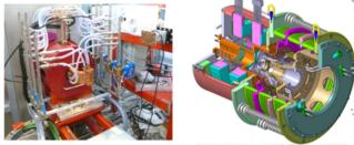
Figure 7: Picture and 3D view of the Spiral 2 ion source with coils and initial 4 electrode extraction system.
