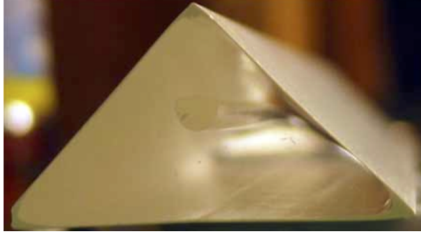
Figure 2.12: A scintillator bar used in PØDule construction. The hole for the WLS-fiber is visible in the center of the triangle.
