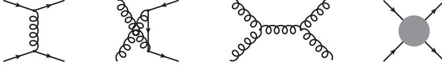
Figure 5.1: Partonic Feynman diagrams contributing to dijet production at tree level. The first three diagrams are SM contributions: t-channel quark scattering, u-channel gluon annihilation into quarks and s-channel gluon scattering. The fourth diagram represents a SMEFT contribution from a four-quark operator.
