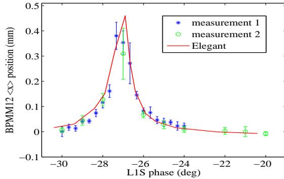
(b) BPMM12 X-position readout after BC1
