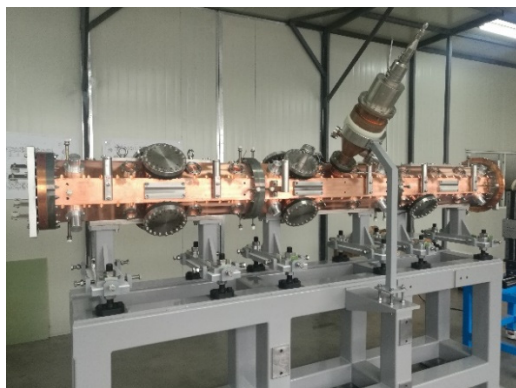
Figure 9: Assembled XiPAF RFQ for the tuning.
