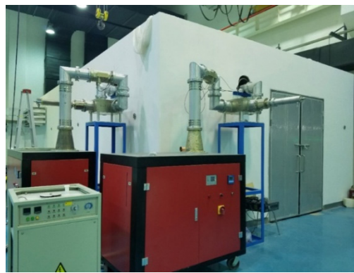
Figure 12: Tetrode-based RF system at site for XiPAF.
