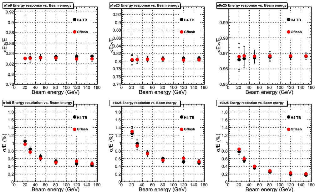
**Figure 2.** The mean energy response (top) and energy resolution (bottom) of  $e^-$  as the beam energy of Gflash (red) and the 2006 test beam data (black).
