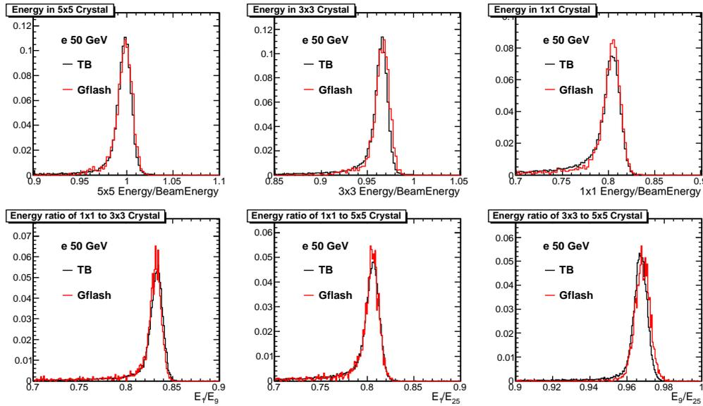
**Figure 1.** The energy response of 50 GeV  $e^-$  of Gflash (red) and the 2006 test beam data (black); the nominal energy response in  $N \times N$  ( $N = 1, 3, 5$ ) crystals (top) and the ratio of  $N \times N$  crystal response (bottom)
