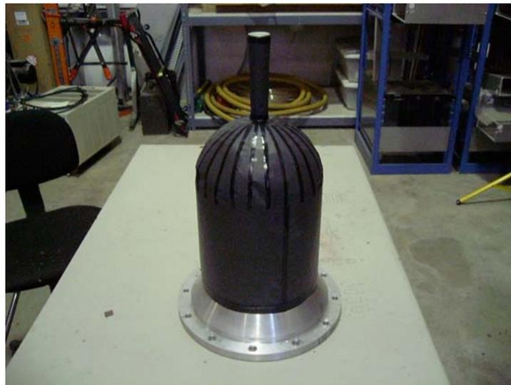
Figure 2-15. A photograph of the foam vacuum chamber that surrounded the whole target system.
