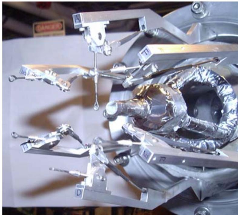
Figure 2-11. The full double-target assembly, showing one solid target inserted, five solid targets retracted, and the thermally insulated cryotarget cell.
