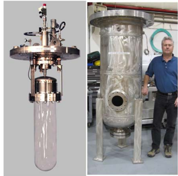
Figure 6. Images from a new 60 kg COUPP bubble chamber under construction at Fermilab.
