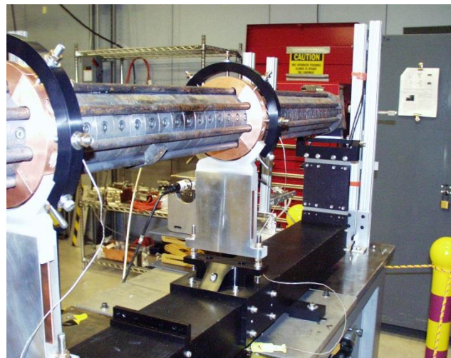
Figure 4: Halo adjuster and saddle used to straighten APS accelerating structures
