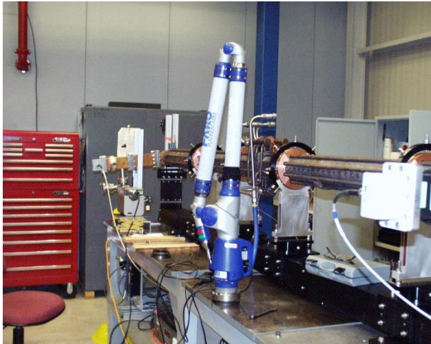
Figure 2: PCMM arm set up to measure an accelerating structure
