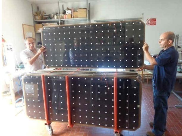
FIGURE 8.1: Gas gaps being made in Italy.
