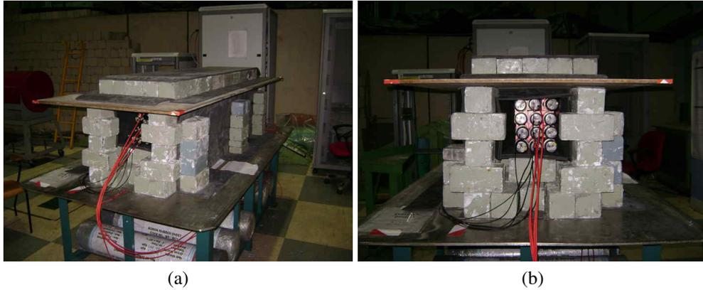
FIGURE 6.3: The current setup with 12 plastic scintillator bars, lead and borated rubber shielding
